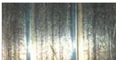
A clean drive roll surface. If particulate debris builds up it can be carried into the gun with the welding wire and cause feed inconsistencies or wire burnbacks in the tip.
